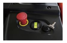
Multi-function LCD instrument shows the battery power, alarm, fault code, running time and speed information, etc.
