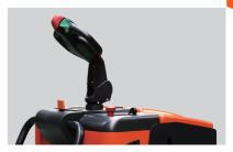
A variety of security measures such as emergency button, reverse button on tiller, and tiller push emergency stop ensure the operator's safety.
