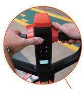
The function of driving with tiller in the **vertical position** helps with work in confined area without sacrificing of safety.
