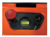
Battery deep discharge protection device, voltage discharge indicator with low voltage automatic cutting and lifting function, for higher battery lifetime.
