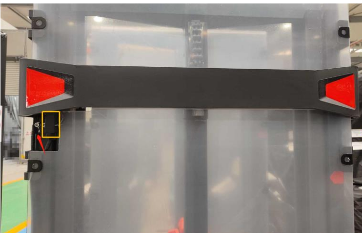
3) The red arrow indicates the 1800mm fork lifting reduction switch-SH (The circuit diagram corresponds to the switch)
