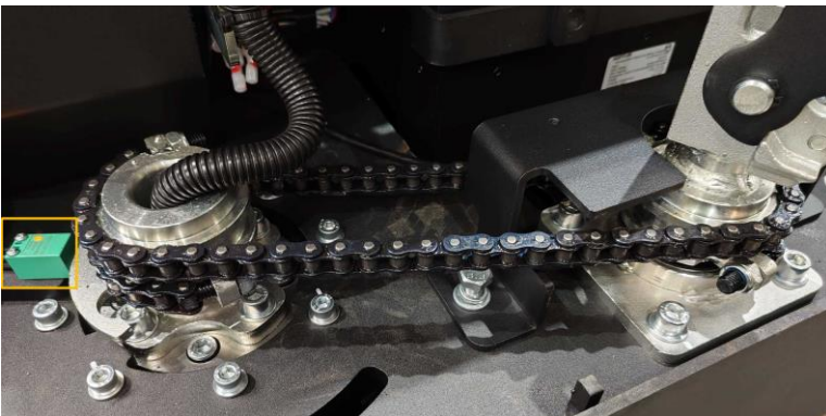
2) Sensor of speed reduction on curve-SC (The circuit diagram corresponds to the switch)
