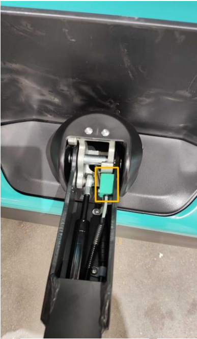
1) Inter-lock switch-SA (The circuit diagram corresponds to the switch)
