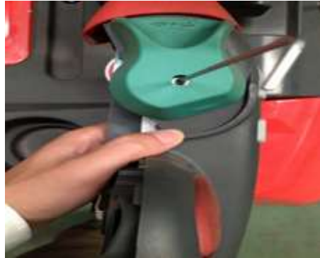
3: loose bolt and remove accelerator cover
