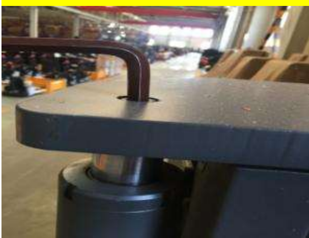
3.Remove the fixed bolt on the upside of cylinder
