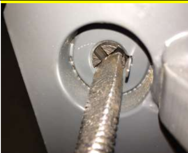
2. Use screwdriver to take out of bolt
