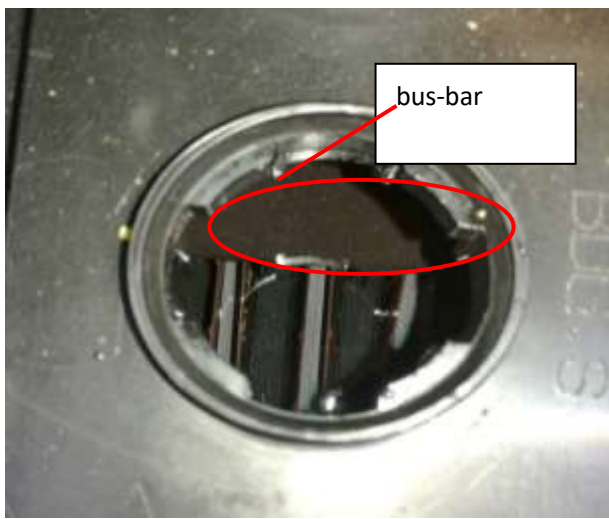
3. Electrolyte level is lower than bus-bar, then add distill water
