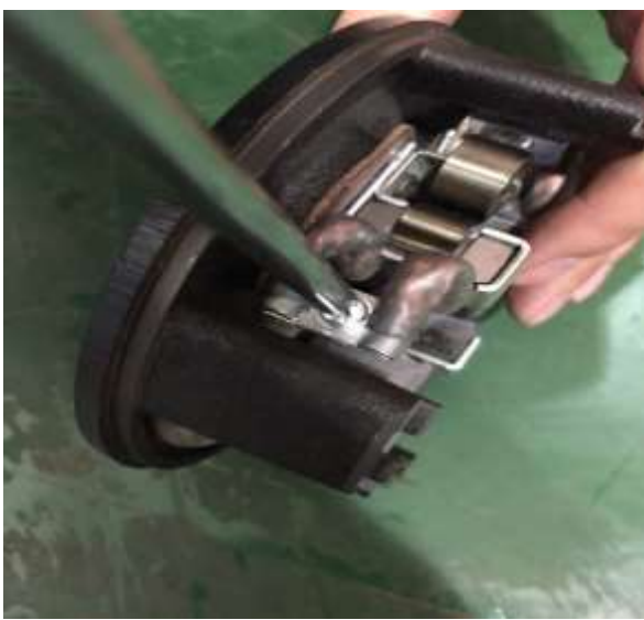
4. Unscrew the screw with a cross screwdriver and take out the carbon brush and replace it. Installation process and the inverse process of the above process.
