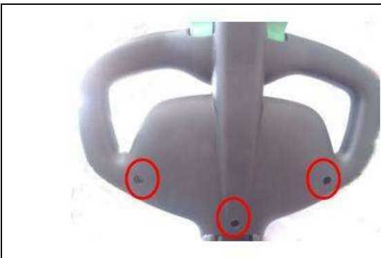
1: loose bolt and remove back cover
