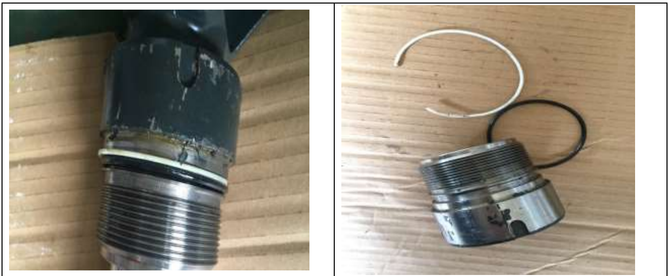
4. Remove dustproof seal and shield ring and Y-type seal
