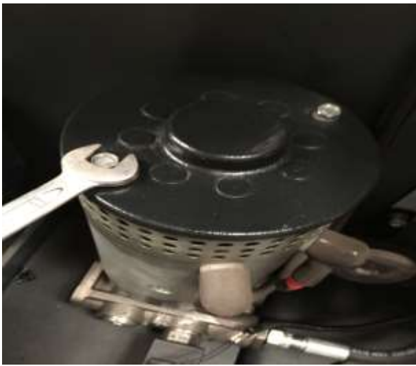
1. Unscrew the bolt with a 10mm open wrench
