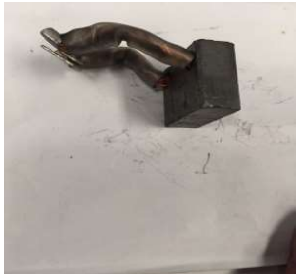
4. Unscrew the screw with a cross screwdriver and take out the carbon brush and replace it. Installation process and the inverse process of the above process.
