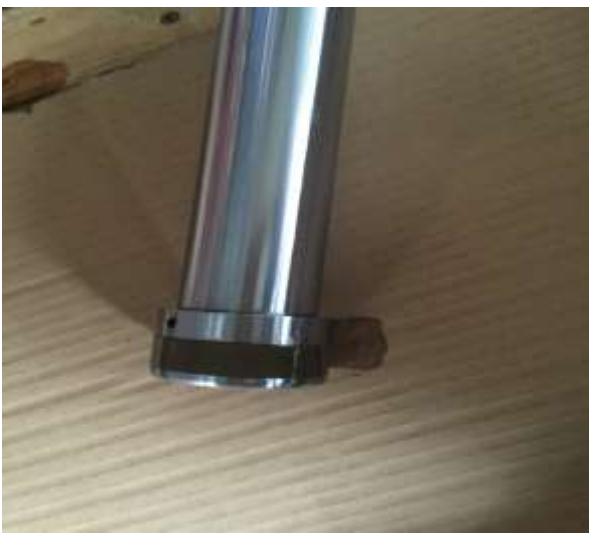
2. Remove piston, then remove retaining ring
