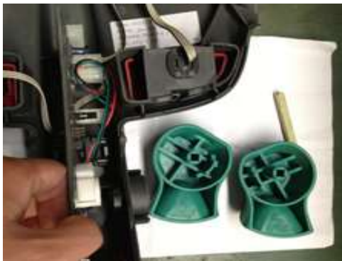
4: Remove the switch shaft
