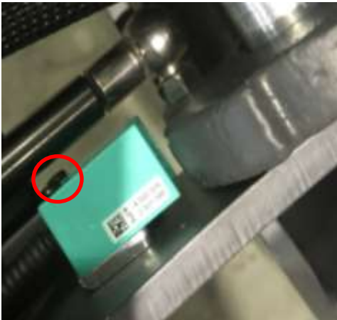
2. Loose bolt , then remove gas spring
