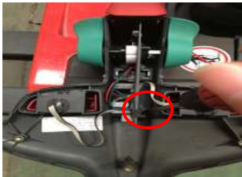
5.remove the bolts ,take out connector and replace the board.
