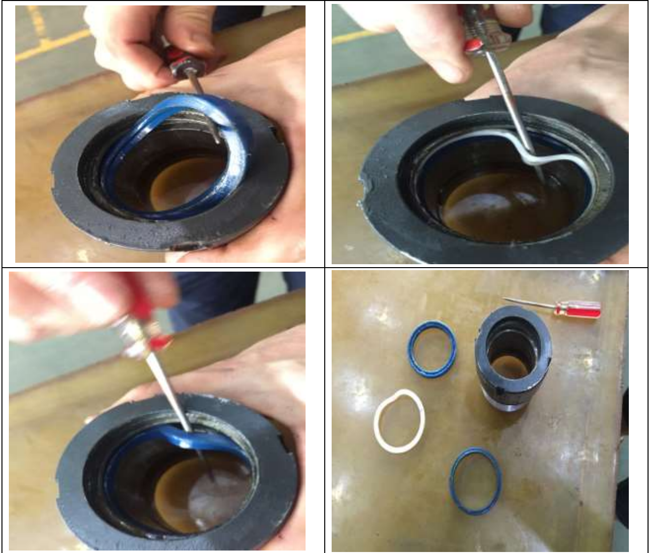
4. Remove dustproof seal and shield ring and Y-type seal
