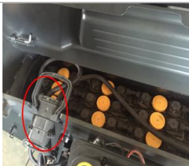
1. Unplug battery switch
