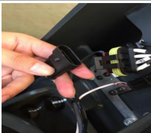
5. Separate the plug,
