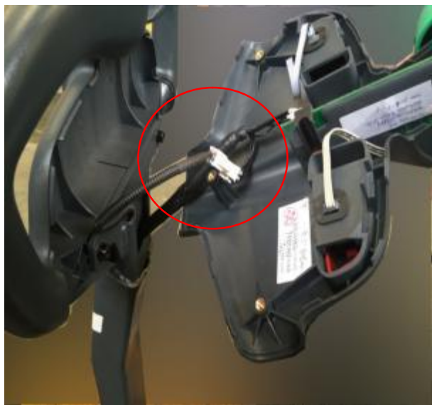
3. Open the handle housing
