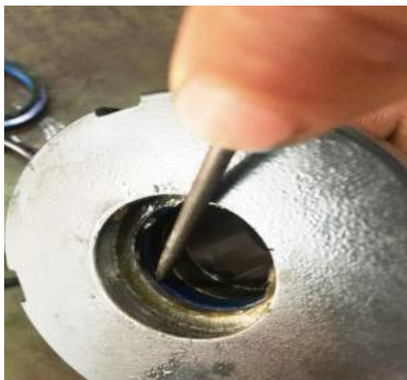
4. Take out sealing ring used for shaft
