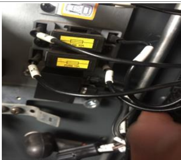
4. Unplug the plug and write down the line number. The position of the line number is shown in the table on the right
