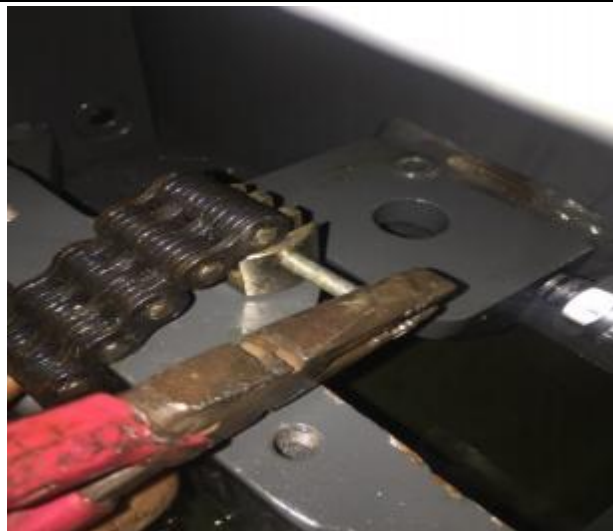
5. Take out the pin shaft
