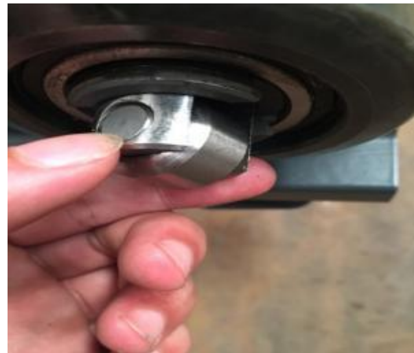
2. Remove the gasket
