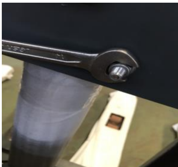
5. Unscrew the hoop bolt with a 13mm open wrench and take the hoop
