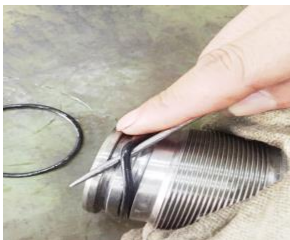
3. Use a screwdriver to remove the dust ring
