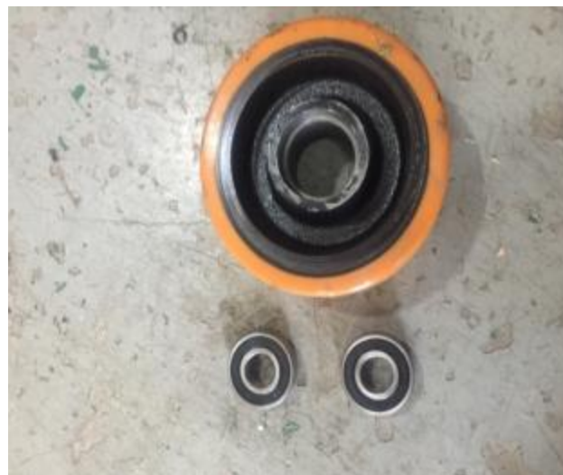
3. When the axle is removed, the axle and other components of the wheel group can be replaced. The installation process is the reverse process of disassembly
