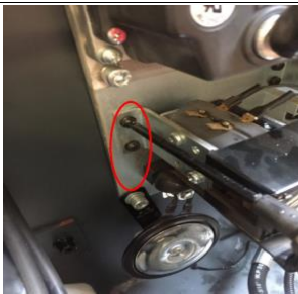
6. Unscrew the two screws with a cross screwdriver
