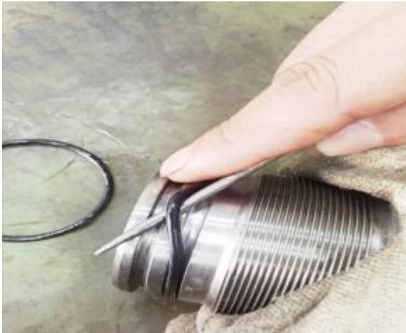
5. Use a small screwdriver to take out the new O-ring,
