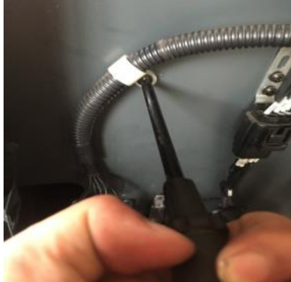
14. Unscrew the wire harness holder with a 14mm cross screwdriver
