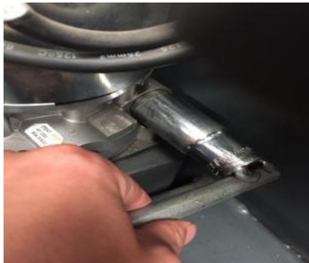
4. Tighten bolts with a 24 mm hexagon socket wrench
