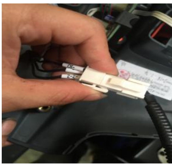
4. Unplug the connector (pay attention to the harness number)
