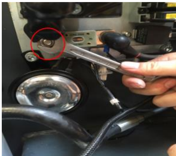
4. Unscrew the bolt with a 13mm open end wrench
