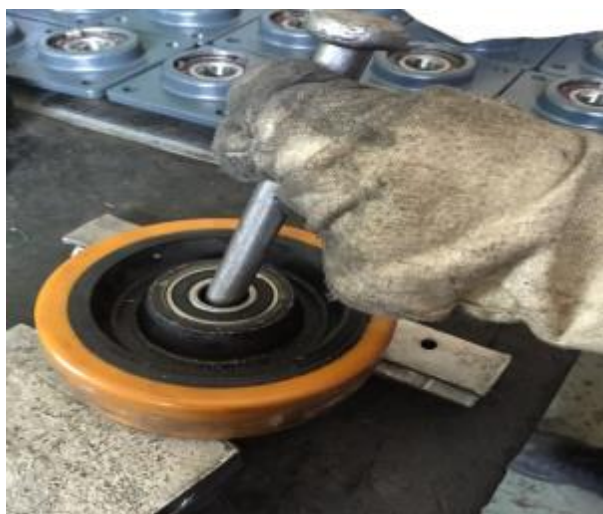
2. Punch the axle out
