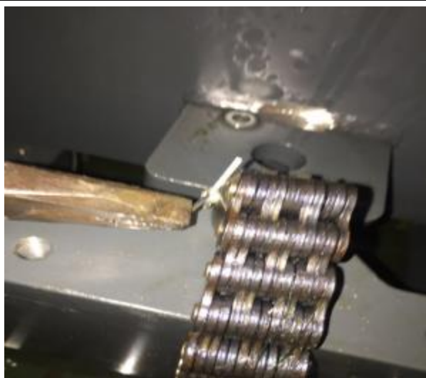
4. Take out the split pin at the bottom of the chain
