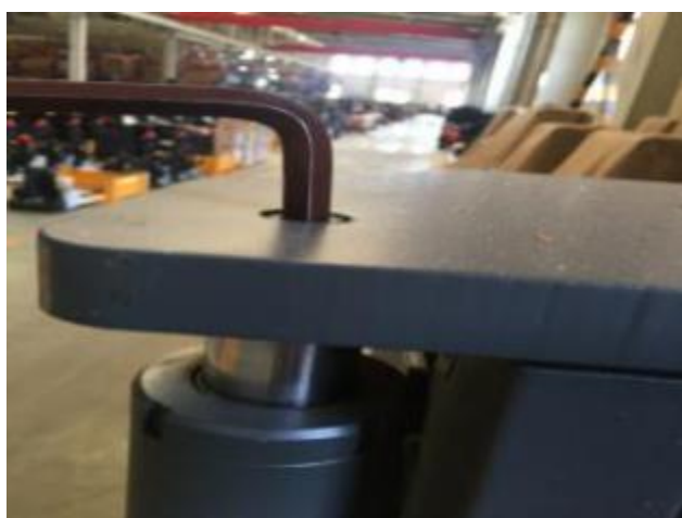
3. Unscrew the fixing bolt at the top of the oil cylinder with a 12mm inner hexagon wrench
