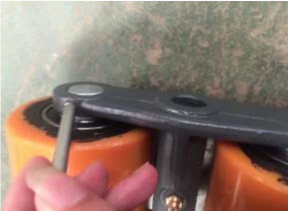
5. Take out the elastic pin with punch
