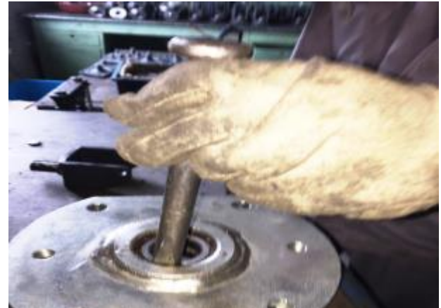
4. Take out both axles with punch.
