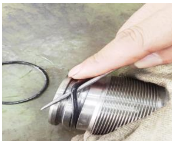
2. Remove the new o-ring with a small screwdriver
