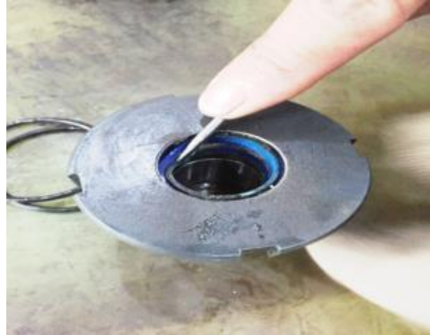
6. Take out the dust ring with a screwdriver
