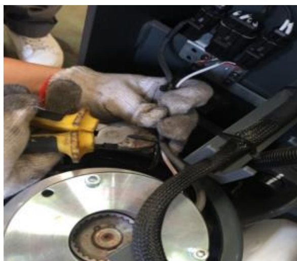
6. Use diagonal pliers to cut the tie that binds the wire harness.
