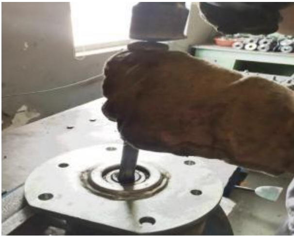
2. Remove the wheel frame with punch
