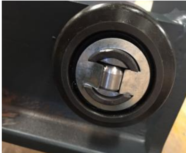
2. Remove the gasket
