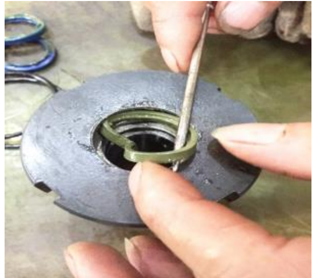
8. Take out the stepseal, the cylinder head sealing ring can be disassembled and replaced
