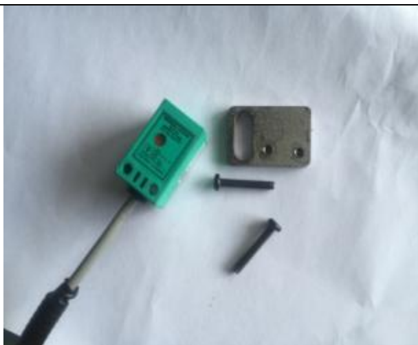
7. The interlock switch can be replaced
