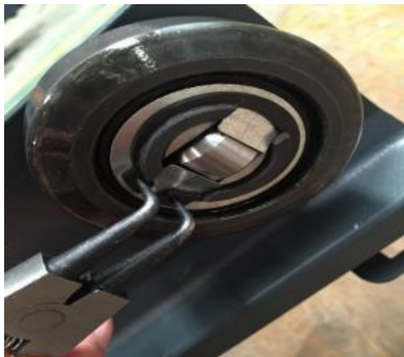
1. Remove the snap spring with the snap pliers
