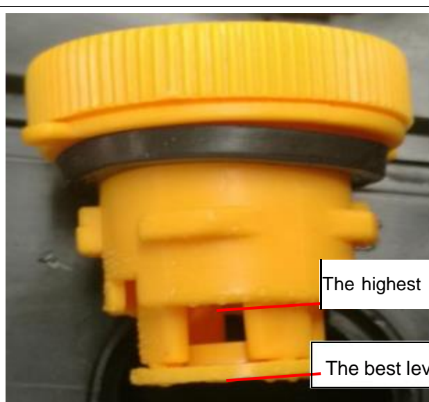
4. Some models of battery add liquid hole can not see the bus drain, liquid level drops to 10mm away from the battery separator, water replenishment
