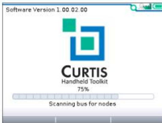
(1) 1313 HHP startup-scan of CANbus for devices
