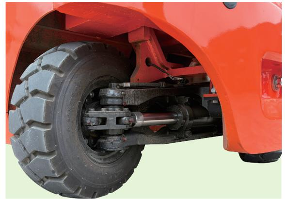
Cast steering axle with large steering cylinder ensures smoother turning.
